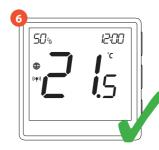
Both devices have been successfully linked. Thermostat displays the main screen, icon " $((\mathbf{P}))$ " appeared on the screen indicating connection with the receiver (EGRFWC in this case).
