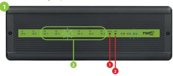
In order to correctly link thermostat with the control box, first select the zone in the control box with the SELECT button (1) (zone which you want to link with thermostat). The LED (2) will flash 3 times for the selected zone. Confirm your selection by clicking PAIR button (2). The LED (2) will flash green with the previously selected zone - binding process has started, it is active for 10 minutes and during this time you can link thermostat with the selected zone.
