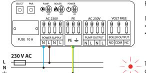
Power supply for wiring centre is  $230 \text{ V} \sim 50 \text{Hz}$ .
