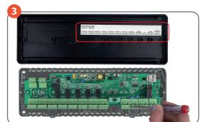
Connect the wires in accordance with the connection description. Refer to the sticker under the top cover.
