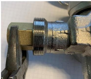
Fit this part into the other side of the mixing valve and tighten using the brass hex tool
