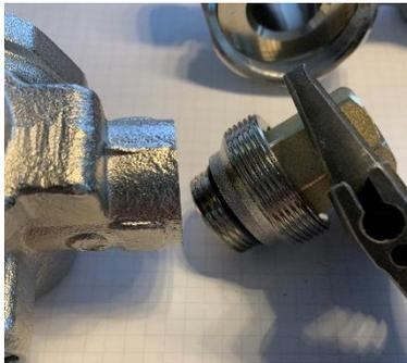
Using the brass hex tool, remove the part from the mixing valve as shown. You may need another pair of grips to hold the body of the mixing valve. There are flats on the body to grip, be careful not to damage any part.
