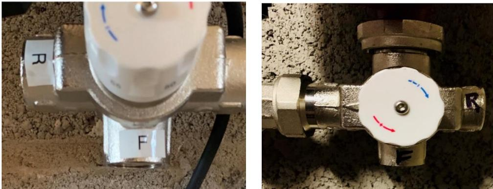
The female connections are 3/4" BSP and fittings are widely available for 22mm and 28mm copper. These are often referred to as 'male/iron' or 'number 3' fittings. Please refer to our technical details in this document for the correct pipe size to use.
